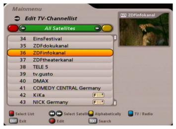
When the menu is called up, the standard setting is for the receiver to show the "All Satellites" channel list with all channels available on the satellites that are being received.
